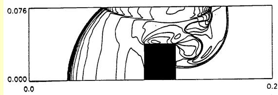
Calculated density map based on a detailed hydrogen combustion mechanism (9 variables)
